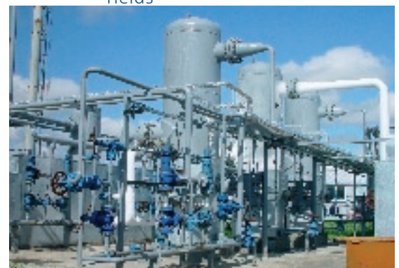
| photo 17 | Compact complex gas treatment plant for small gas-condensate fields
